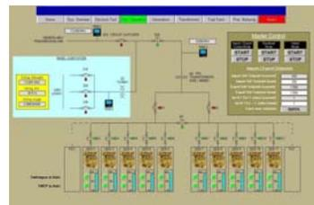
Supervisory Control and Data Acquisition (SCADA) systems. Remote equipment monitoring.
